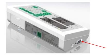
Plug the cable to the printer, and then connect its 9D connector to the indicator.
