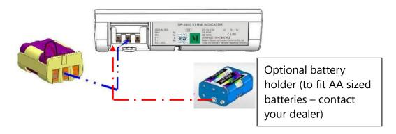
4. Place the housing back in the back of the indicator, and close the battery housing cover.
