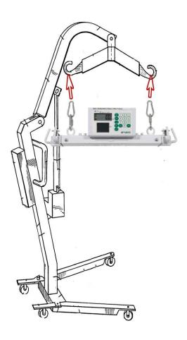
2. Place the patient properly in the sling and attach sling loops onto the hooks on both sides of M-600 / M-605. The design and procedure may vary depending on the different sling makers. Please base on the instructions of the sling product.
